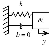
FIGURE 1. One-mass vibration model.
