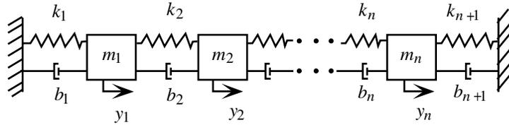
FIGURE 2. Multi-mass vibration model.
