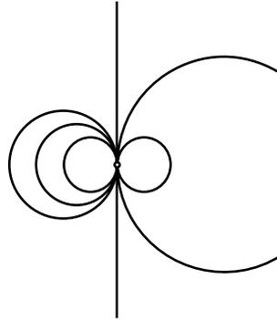
FIGURE 3. Parabolic pencil.
