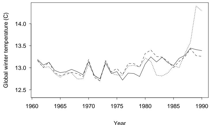
FIG. 1. Global average “winter” temperature ( $^{\circ}\text{C}$ ) series by three estimation methods. Solid lines: SS-ANOVA estimates, that is,  $d_1 + d_2\phi(t) + g_1(t)$  in (2); dotted lines: annual averages of raw data; dashed lines: annual averages of anomalies. The series by the anomaly approach is shifted up by an (estimated) grand average, that is,  $d_1$  in (2), to match other two series.
