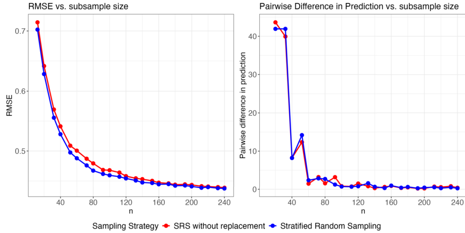
Figure 4.4: We plot the RMSE (left panel) and pairwise difference in predictions (right panel) over different subsample size under SRS without replacement (red) and stratified random sampling (blue). The elbow of pairwise difference in predictions is much sharper in both sampling designs.
