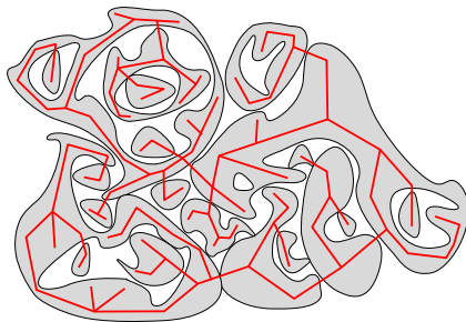
FIG. 1. The MST connects the percolation p -clusters without creating cycles, yielding the cluster-tree \text{MST}^p .
