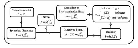
FIG. 1. Block diagram of antipodal chaos shift-keying communication systems in both the coherent and non-coherent forms. In the coherent form, the reference signal is known exactly at the receiver, and in the non-coherent form it is known inexactly at the receiver by transmission or synchronization.
