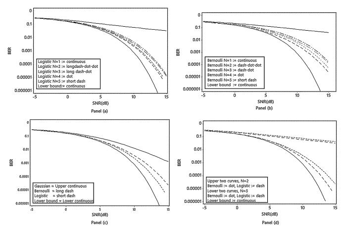
FIG. 2. BER plotted against SNR<sub>db</sub> for antipodal CSK; order of curves from panel variables; solid lowest curve in each panel is the BER Jensen lower bound. Panel (a): logistic map spreading, spreading factors N = 1, 2, ..., 5. Panel (b): Bernoulli-shift map spreading, spreading factors N = 1, 2, ..., 5. Panel (c): Bernoulli-shift, logistic and Gaussian spreading, spreading factor N = 5. Panel (d): Bernoulli-shift and logistic spreading, spreading factor N = 5.
