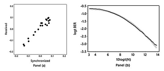
FIG. 7. Panel (a): Scatterplot of a received message segment and its synchronized version for N = 20 spreading. Panel (b): BER curves of the experimental non-coherent shift-keying communication system (light curve) and of the corresponding coherent system (dark curve) in which there is no synchronization error.
