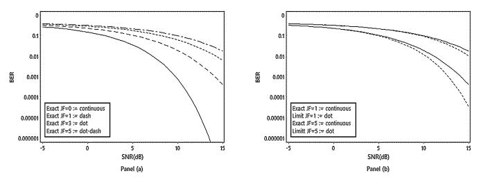
FIG. 5. Wide band on-off pulsed jamming of coherent CSK with logistic spreading, spreading factor N = 4 and jamming number M = 2. Panel (a): Exact BER curves for the coherent lower bound and jamming factors JF = 0, 1, 3, 5. Panel (b): Comparison of limiting and exact BER curves for jamming factors JF = 1, 5.
