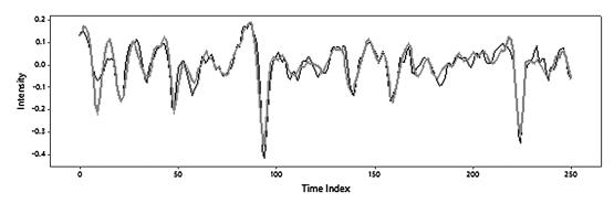
FIG. 6. Comparison at 250 time points of a laser generated chaotic wave (thin black line) and its remotely synchronized version (thick grey line) from an experimental CSK communication system.
