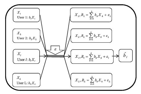
FIG. 8. Block diagram of an antipodal multi-user coherent CSK communication system and transmission by the active lth user.
