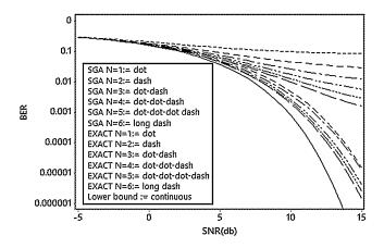
FIG. 3. Comparison of using the exact BER result for the lower set of curves with using the SGA approach for the upper set of curves, for coherent CSK with logistic map spreading, spreading factors N = 2, 3, ..., 6, and the lower bound.
