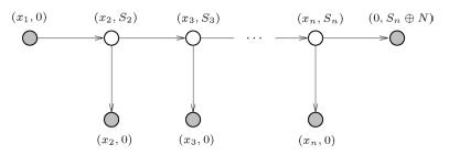
FIG. 1. Hidden Markov model for noisy parity. The model computes  $N \oplus \bigoplus_{i \in T} x_i$ , where the  $x_i$ 's are uniform over  $\{0, 1\}$ , T is a subset of  $\{1, ..., n\}$ , and N is a small random noise. The  $S_i = \bigoplus_{j \in T, j \leq i} x_j$  are the partial sums over variables included in T. The observed nodes are in light gray. The hardness proof follows from a standard reduction technique similar to that used in [22].
