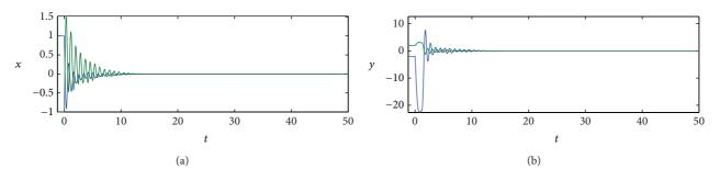
FIGURE 2: State trajectory of the system with  $\rho_1 = \rho_2 = 0.13$  for Example 7 with two nodes.
