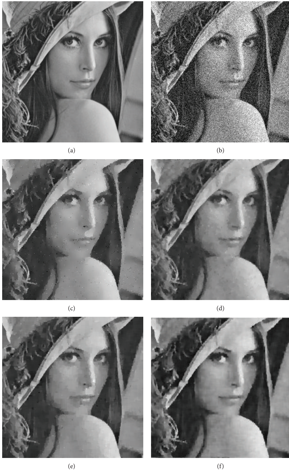
FIGURE 2: Lena image ( 300 \times 300 ). (a) Original image. (b) Noisy image corrupted by Gaussian noise for \sigma = 30 . (c) PM algorithm, K = 5 , \tau = 0.25 (113 steps). (d) TV method, \tau = 0.25 (129 steps). (e) Our method, K = 0.1 , \tau = 5 (15 steps). (f) D- \alpha -PM algorithm, K = 4 , \tau = 2 (10 steps).
