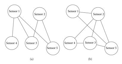
FIGURE 1: Two topology structures of WiNCS.
