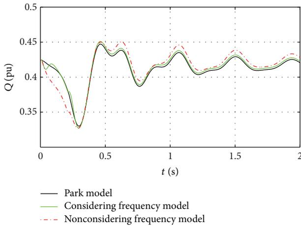
FIGURE 13: Reactive power of induction motor.
