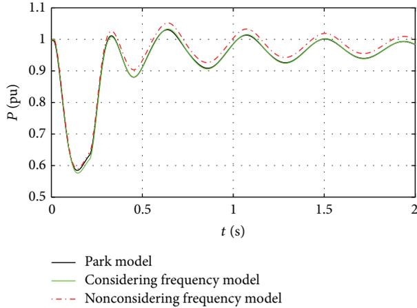
FIGURE 12: Active power of induction motor.
