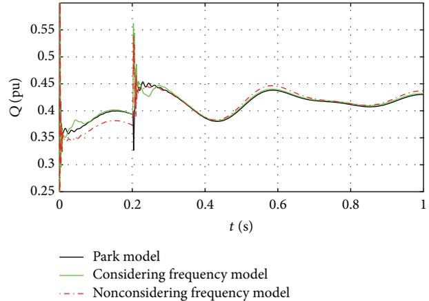
FIGURE 7: Reactive power of induction motor.
