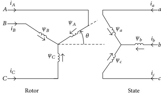
FIGURE 1: Stator and rotor circuits of an induction motor.
