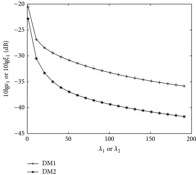
FIGURE 4: The relationship between the optimal Lagrange multiplier  $\lambda_1$  ( $\lambda_2$ ) and the stopband attenuation  $\varepsilon_1$  (the passband fidelity  $\xi_1$ ), in which the filters were designed by DM1 (DM2).
