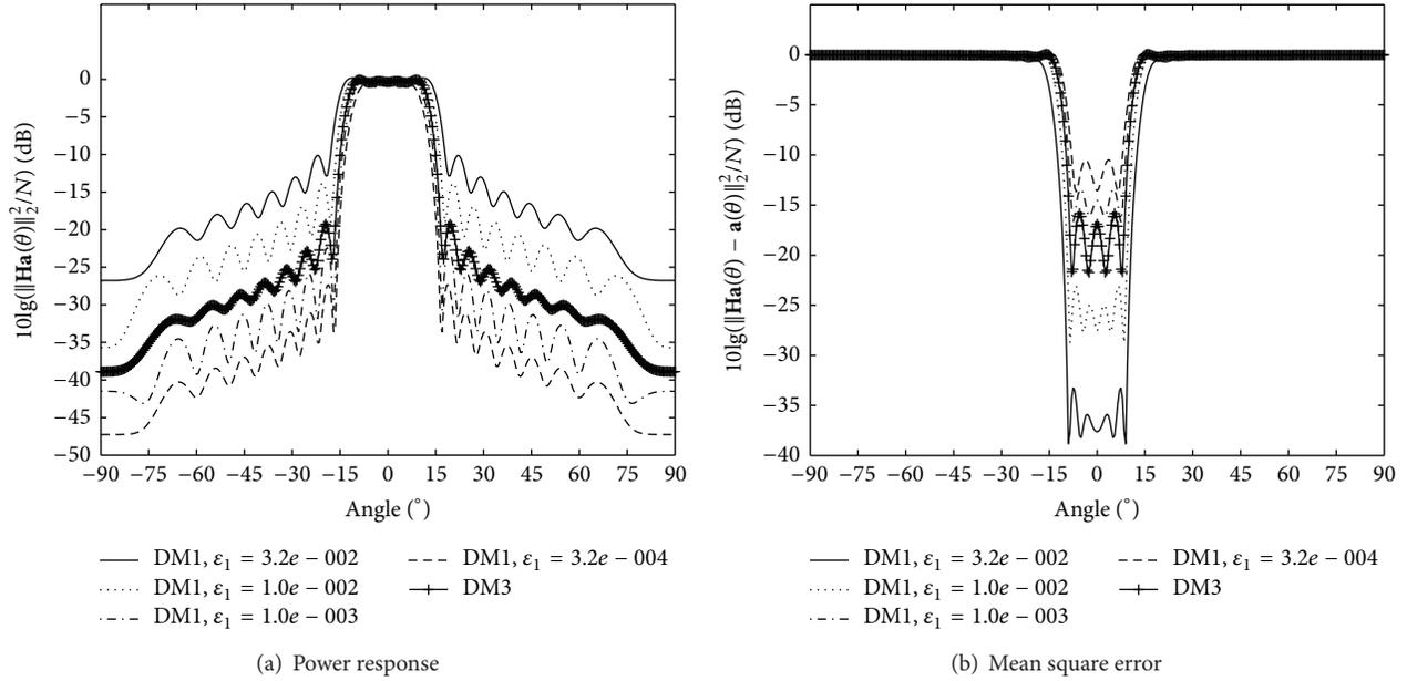
FIGURE 1: Characteristics of the spatial matrix filters designed by DM1 and DM3.
