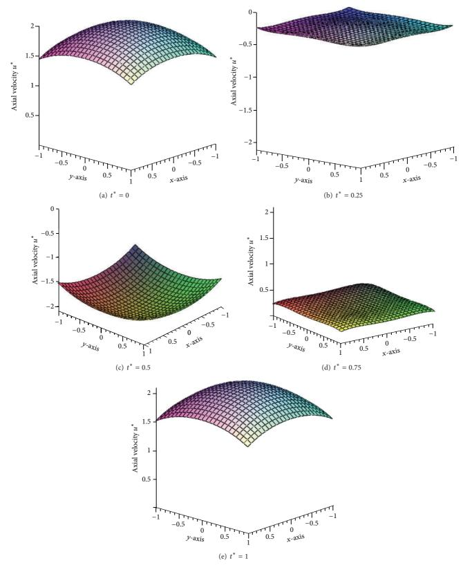
FIGURE 6: Axial velocity profile on the cross-section of the channel with the area of  $1.0 \times 10^{-6}$  m<sup>2</sup> and ratio b/a = 1 under the frequency  $\omega = \alpha/\rho a^2$  with  $\alpha = 0.005$  and slip length of 0.001 for various instants of time.
