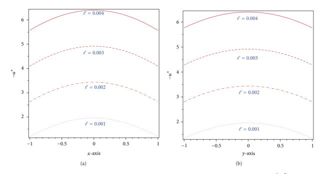
FIGURE 4: 2D velocity profile along the *x*-axis and *y*-axis on the cross-section of the channel with the area of  $1.0 \times 10^{-6}$  m<sup>2</sup> and ratio  $\varepsilon$  of 3/4 for constant pressure gradient under different slip lengths  $\ell$  values.
