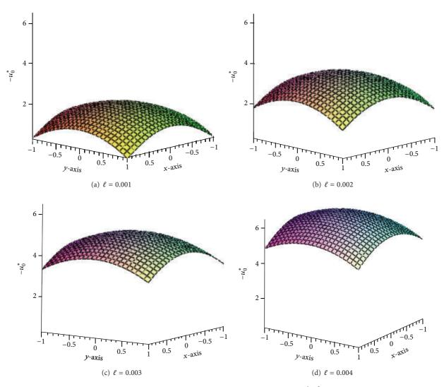
FIGURE 3: Axial velocity profile on the cross-section of the channel with the area of  $1.0 \times 10^{-6}$  m<sup>2</sup> and ratio  $\varepsilon$  of 3/4 for constant pressure gradient under various values of slip lengths  $\ell$ : (a)  $\ell$  = 0.001; (b)  $\ell$  = 0.002; (c)  $\ell$  = 0.003; (d)  $\ell$  = 0.004.
