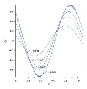
FIGURE 8: Influence of slip length on the flow rate  $Q_1^*$  on the crosssection of the channel with the area of  $1.0 \times 10^{-6}$  m<sup>2</sup> and ratio b/a of 1 under the frequency  $\omega = \alpha/\rho a^2$  with  $\alpha = 0.005$  at various instants of time.
