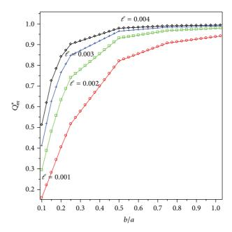
FIGURE 10: Influence of ratio  $\varepsilon$  of b/a and slip length  $\ell$  on the amplitude of the flow rate on the cross-section of the channel with constant area of  $1.0 \times 10^{-6}$  m<sup>2</sup> under the frequency  $\omega = \alpha/\rho a^2$  with  $\alpha = 0.005$ .
