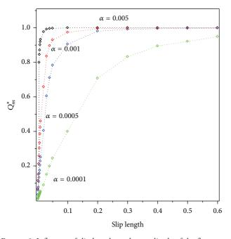
FIGURE 9: Influence of slip length on the amplitude of the flow rate  $Q_m^*$  on the cross-section of the channel with the area of  $1.0 \times 10^{-6}$  m<sup>2</sup> and ratio b/a of 1 under different frequencies  $\omega = \alpha/\rho a^2$  with different  $\alpha$ .
