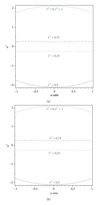
FIGURE 7: Axial velocity along the *x*-axis and *y*-axis on the crosssection of the channel with the area of  $1.0 \times 10^{-6}$  m<sup>2</sup> and ratio b/a =1 under the frequency  $\omega = \alpha/\rho a^2$  with  $\alpha = 0.005$  and slip length of 0.001 at various instants of time.
