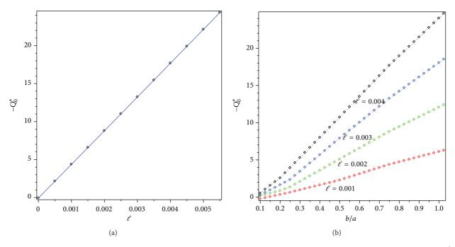
FIGURE 5: Influence of slip length and the ratio  $\varepsilon$  on the flow rate  $Q_0^*$  on the cross-section of the channel with the constant area of  $1.0 \times 10^{-6}$  m<sup>2</sup> for a constant gradient pressure.
