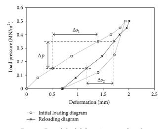
FIGURE 1: Example load-deformation curves for soil.
