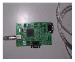
FIGURE 7: CAN card in the test.
