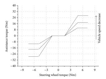
FIGURE 8: Linear assistant characteristics in the test.
