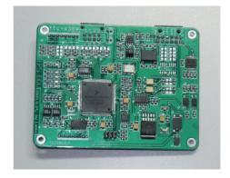
FIGURE 4: EPS controller for the test.
