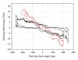
FIGURE 9: Steering wheel torque in the basic assist strategy in the test.
