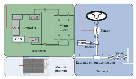
FIGURE 1: Overall view of the developed test rig.
