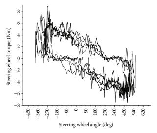
FIGURE 12: The relationship between the steering wheel torque and the steering wheel angle in the basic control.
