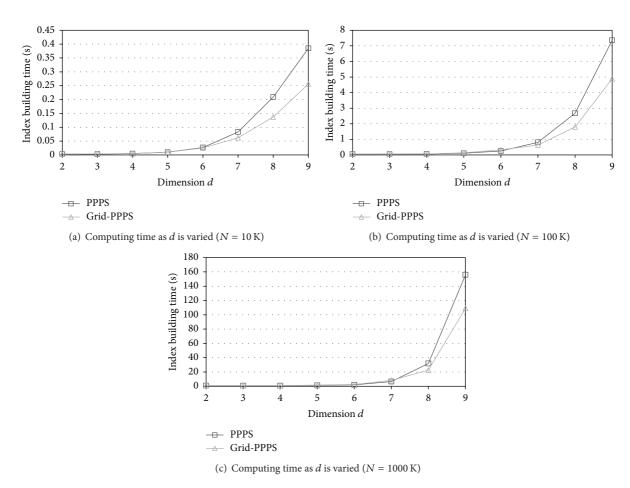
FIGURE 6: The comparison of the computing time of the Grid-PPPS and PPPS as d and N are varied related to Experiment 2.
