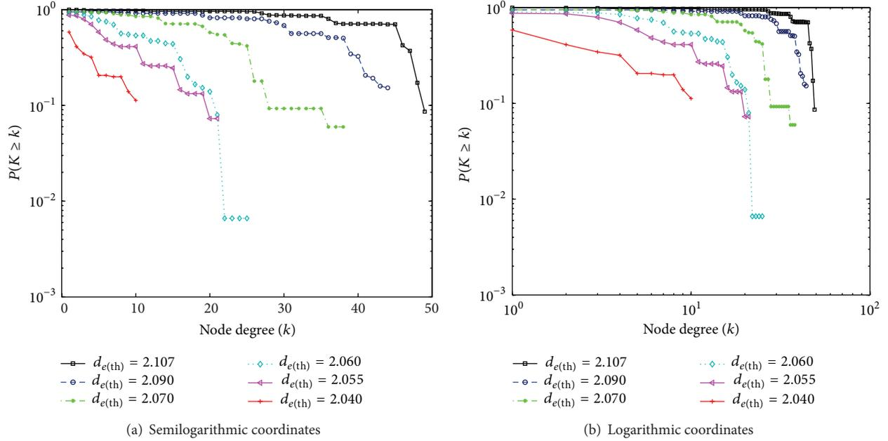
FIGURE 8: Cumulative degree distribution of electrical distance-based network model of TJ220 Grid.
