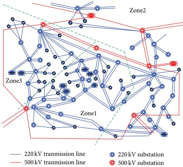
FIGURE 3: Geographical wiring layout of TJ220 Grid.
