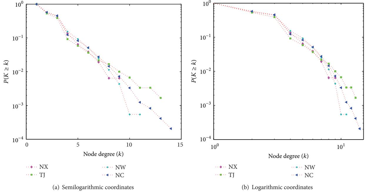
FIGURE 1: Cumulative degree distribution of topology-based model of power grids.
