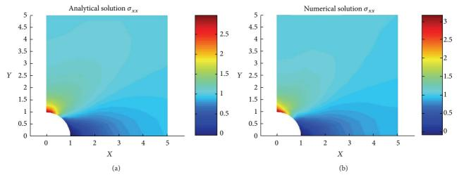
FIGURE 13: Stress  $\sigma_x$ : analytical results (a) and RGD numerical results (b).
