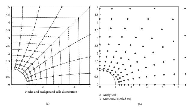
FIGURE 12: Plate with a central circular hole: (a) 99 nodes' distribution, (b) analytical and RGD solution of displacement.
