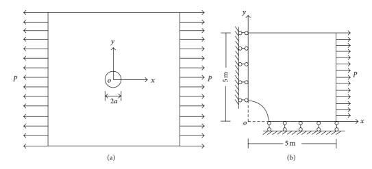
FIGURE 11: Plate with a central circular hole and its model problem: (a) a plate with a hole, (b) a quarter of the plate and boundary conditions.
