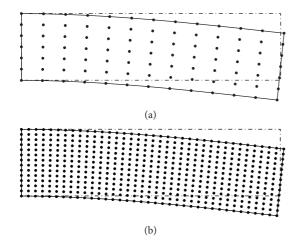
FIGURE 7: Displacement  $13 \times 7$  (a) and  $36 \times 13$  (b) regular nodes distribution (scaled 400).
