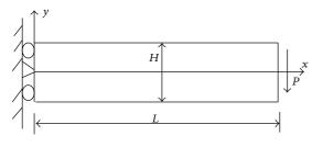
FIGURE 3: Cantilever beam.
