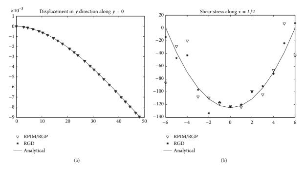
FIGURE 5: Results for 325 irregular nodes: (a) displacement and (b) shear stress.
