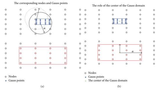
FIGURE 1: The distribution of the nodes and the Gauss points: find the 1-1 mapping (a); assign the 1-1 mapping (b).
