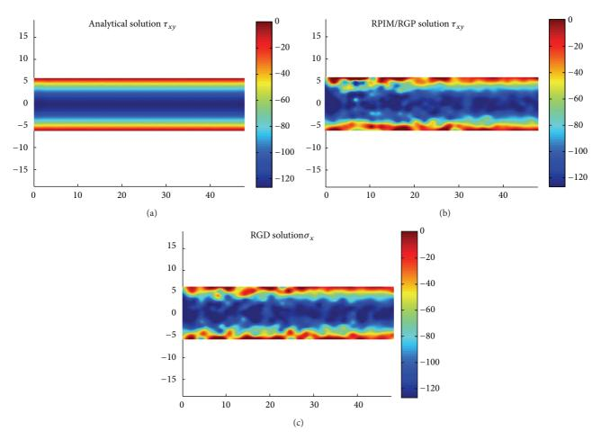
FIGURE 9: Shear stress  $\tau_{xy}$ : analytical results (a), RGP numerical results (b), and RGD numerical results (c).
