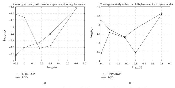
FIGURE 6: Convergence study with error of displacement: regular nodes (a), irregular nodes (b).
