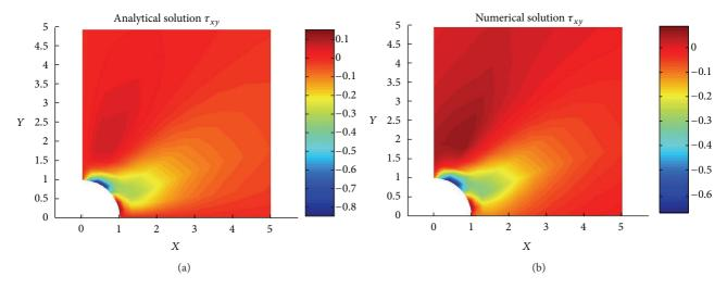
FIGURE 14: Shear stress  $\tau_{xy}$ : analytical results (a) and RGD numerical results (b).
