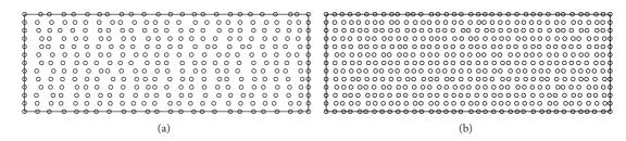
FIGURE 4: Meshless models with irregular data points: 325 nodes (a), 481 nodes (b).
