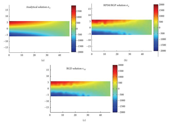
FIGURE 8: Stress  $\sigma_x$ : analytical results (a), RGP numerical results (b), and RGD numerical results (c).
