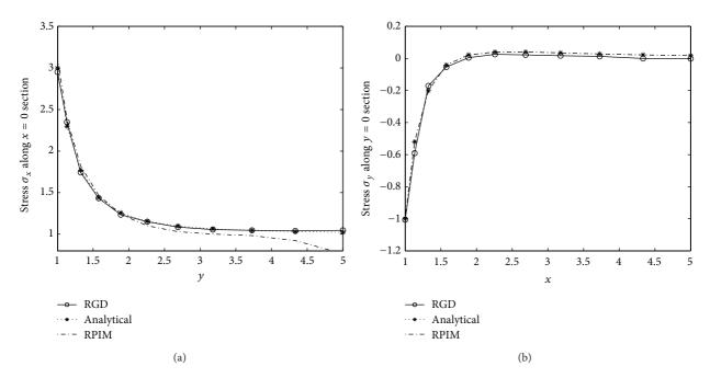
FIGURE 15: Comparisons of RGD and analytical solution: stress  $\sigma_x$  at the stations along the left edge of the plate (a) and stress  $\sigma_y$  at the stations along the bottom edge of the plate (b).
