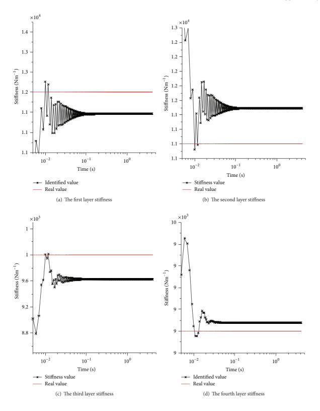
FIGURE 4: Stiffness identification results when SNR is 30.
