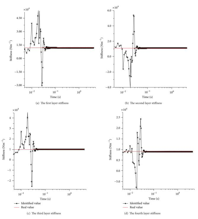
FIGURE 2: Structural stiffness identification result without noise.
