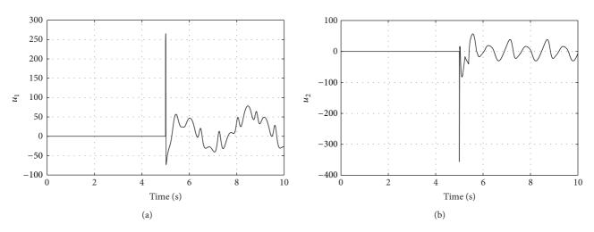
FIGURE 4: Control input using sliding mode control.
