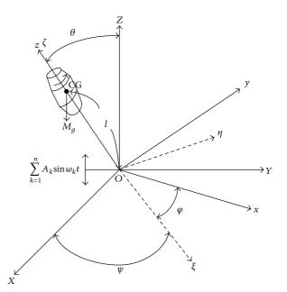
FIGURE 1: A schematic diagram of a heavy symmetric gyroscope [2].
