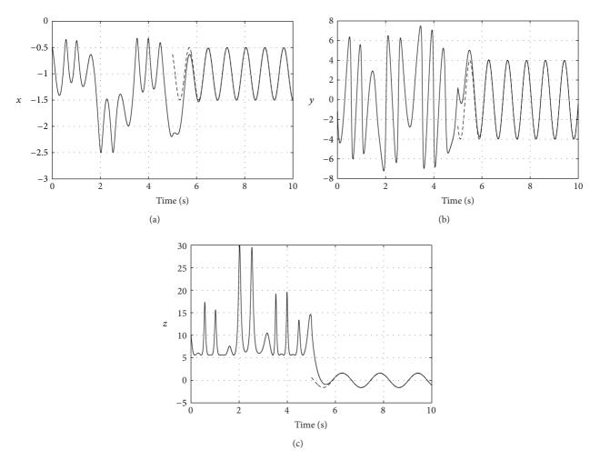
FIGURE 5: Time response of gyroscope via fuzzy sliding mode control.
