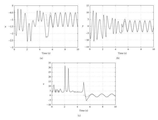
FIGURE 3: Time response of gyroscope via sliding mode control.
