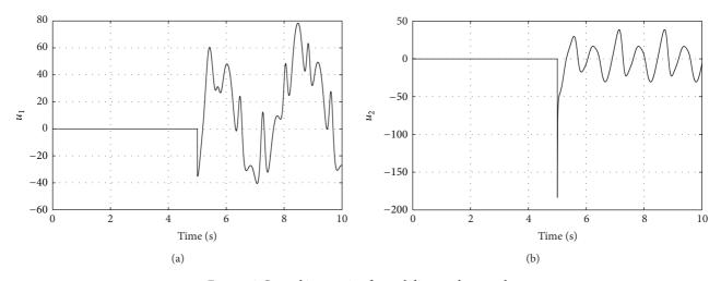
FIGURE 6: Control input using fuzzy sliding mode control.
