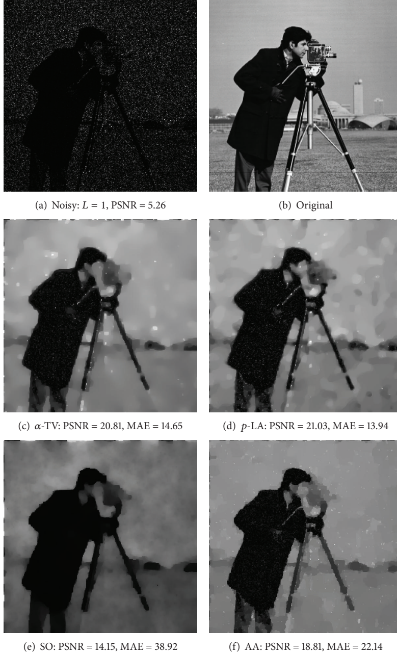
FIGURE 8: Cameraman image ( 512 \times 512 ). (a) Noisy image corrupted by speckle noise for L = 1 in (8). (b) Original image. (c) Our algorithm by \alpha -TV, \sigma = 2 , k = 0.01 , and \tau = 0.05 . (d) Our algorithm by p -LA, p_U = 1.3 . (e) SO algorithm, \lambda = 0.04 , \alpha = 0.25 . (f) AA algorithm, \lambda = 125 .
