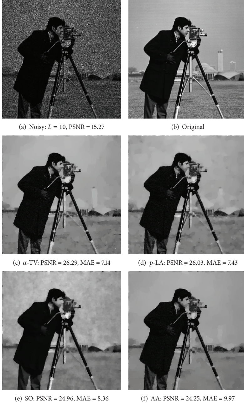
FIGURE 10: Cameraman image ( 512 \times 512 ). (a) Noisy image corrupted by speckle noise for L = 10 in (8). (b) Original image. (c) Our algorithm by \alpha -TV, \sigma = 8/6 , k = 0.005 , and \tau = 0.05 . (d) Our algorithm by p -LA, p_U = 1.2 . (e) SO algorithm, \lambda = 1 , \alpha = 0.25 . (f) AA algorithm, \lambda = 390 .
