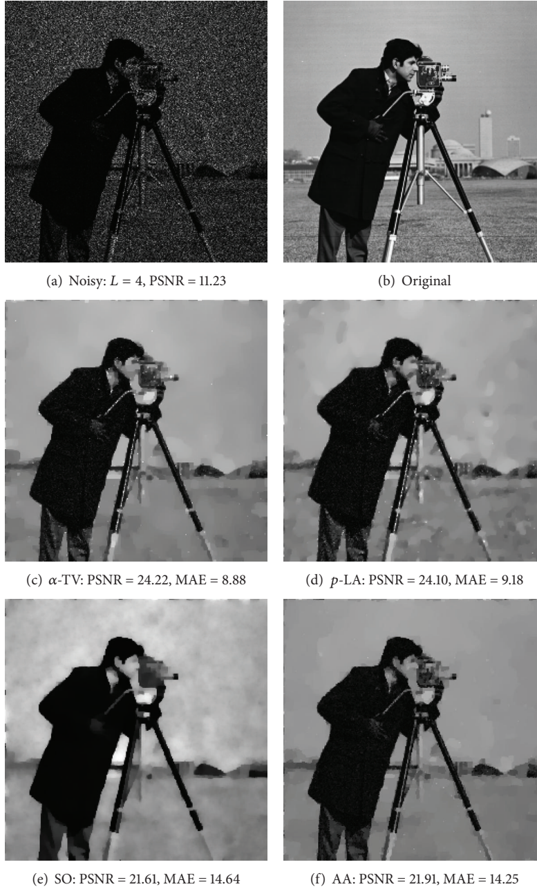
FIGURE 9: Cameraman image ( 512 \times 512 ). (a) Noisy image corrupted by speckle noise for L = 4 in (8). (b) Original image. (c) Our algorithm by \alpha -TV, \sigma = 2 , k = 0.005 , and \tau = 0.05 . (d) Our algorithm by p -LA, p_U = 1.2 . (e) SO algorithm, \lambda = 0.2 , \alpha = 0.25 . (f) AA algorithm, \lambda = 240 .
