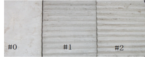
FIGURE 1: The topography of the concrete plate in the test.
