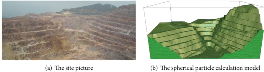
FIGURE 5: The model after excavating.
