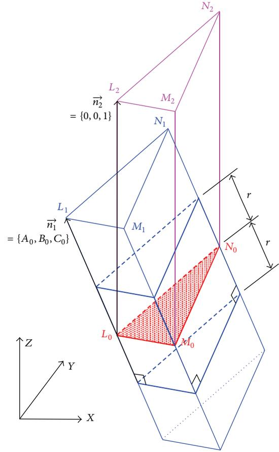
FIGURE 2: Excavating space of a triangular facet.
