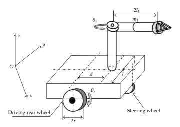
Figure 2: The wheeled mobile manipulator in the simulation.
