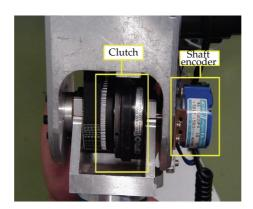
Figure 1: The hybrid joint.
