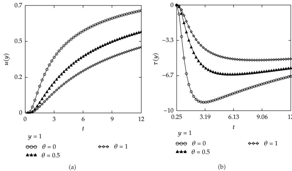
**Figure 3:** Profiles of the velocity field  $u(y,t)$  and the shear stress  $\tau(y,t)$  for fractional Maxwell fluid given by (4.7) and (4.15), for  $U = 1, y = 1, \nu = 0.379, \mu = 33, \lambda = 1.5, \alpha = 0.2$ , and different values of  $\theta$ .
