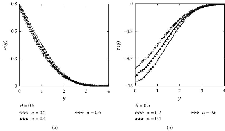
**Figure 7:** Profiles of the velocity field  $u(y,t)$  and the shear stress  $\tau(y,t)$  for fractional Maxwell fluid given by (4.7) and (4.15), for  $U = 1, y = 1, \nu = 0.379, \mu = 33, \lambda = 1.5, \theta = 0.5, t = 5$  s, and different values of  $\alpha$ .
