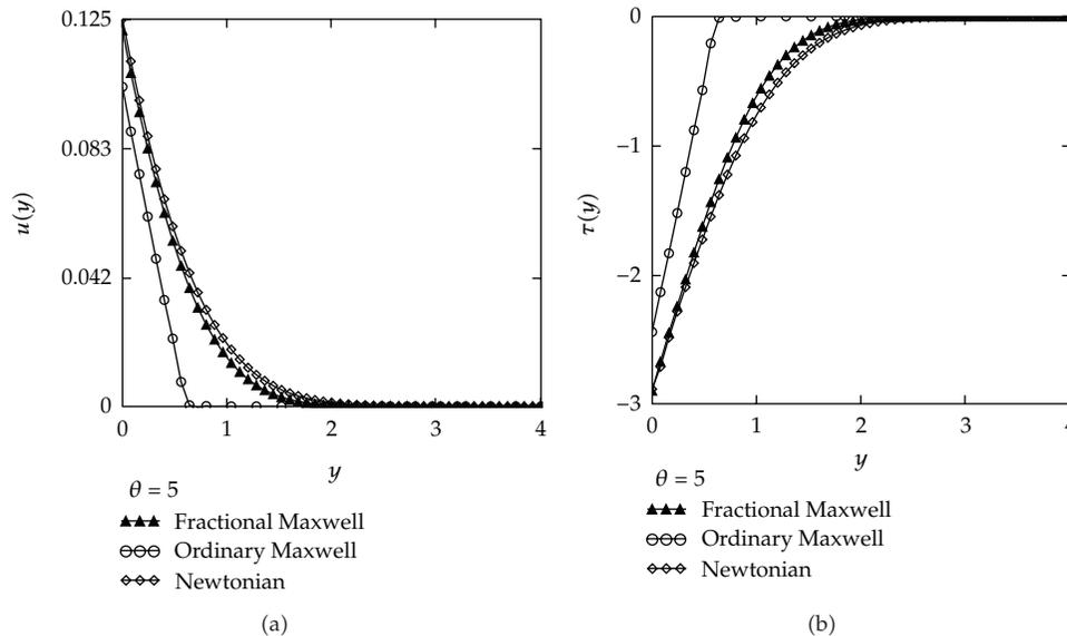
**Figure 14:** Profiles of the velocity field  $u(y,t)$  and the shear stress  $\tau(y,t)$  for fractional Maxwell, ordinary Maxwell and Newtonian fluids, for  $U = 1$ ,  $y = 1$ ,  $\nu = 0.379$ ,  $\mu = 33$ ,  $\lambda = 1.5$ ,  $\alpha = 0.2$ ,  $t = 2$  s, and  $\theta = 5.0$ .
