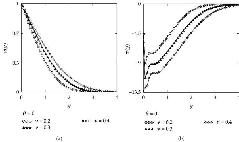
**Figure 10:** Profiles of the velocity field  $u(y,t)$  and the shear stress  $\tau(y,t)$  for fractional Maxwell fluid given by (5.3) and (5.4), for  $U = 1, y = 1, \rho = 87.071, \lambda = 1.5, \alpha = 0.2, \theta = 0.0, t = 5\text{ s}$ , and different values of  $\nu$ .
