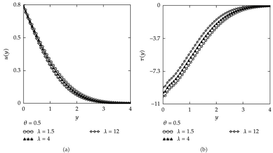
**Figure 5:** Profiles of the velocity field  $u(y,t)$  and the shear stress  $\tau(y,t)$  for fractional Maxwell fluid given by (4.7) and (4.15), for  $U = 1$ ,  $y = 1$ ,  $\nu = 0.379$ ,  $\mu = 33$ ,  $\alpha = 0.2$ ,  $\theta = 0.5$ ,  $t = 5$  s, and different values of  $\lambda$ .
