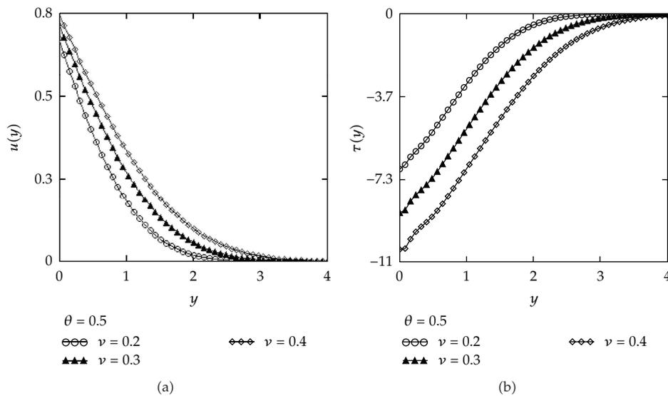
**Figure 9:** Profiles of the velocity field  $u(y,t)$  and the shear stress  $\tau(y,t)$  for fractional Maxwell fluid given by (4.7) and (4.15), for  $U = 1, y = 1, \rho = 87.071, \lambda = 1.5, \alpha = 0.2, \theta = 0.5, t = 5$  s, and different values of  $\nu$ .
