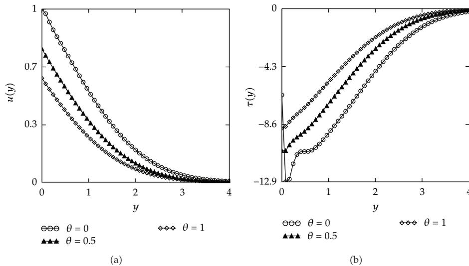
**Figure 11:** Profiles of the velocity field  $u(y,t)$  and the shear stress  $\tau(y,t)$  for fractional Maxwell fluid given by (4.7) and (4.15), for  $U = 1, y = 1, \nu = 0.379, \mu = 33, \lambda = 1.5, \alpha = 0.2, t = 5\text{ s}$ , and different values of  $\theta$ .
