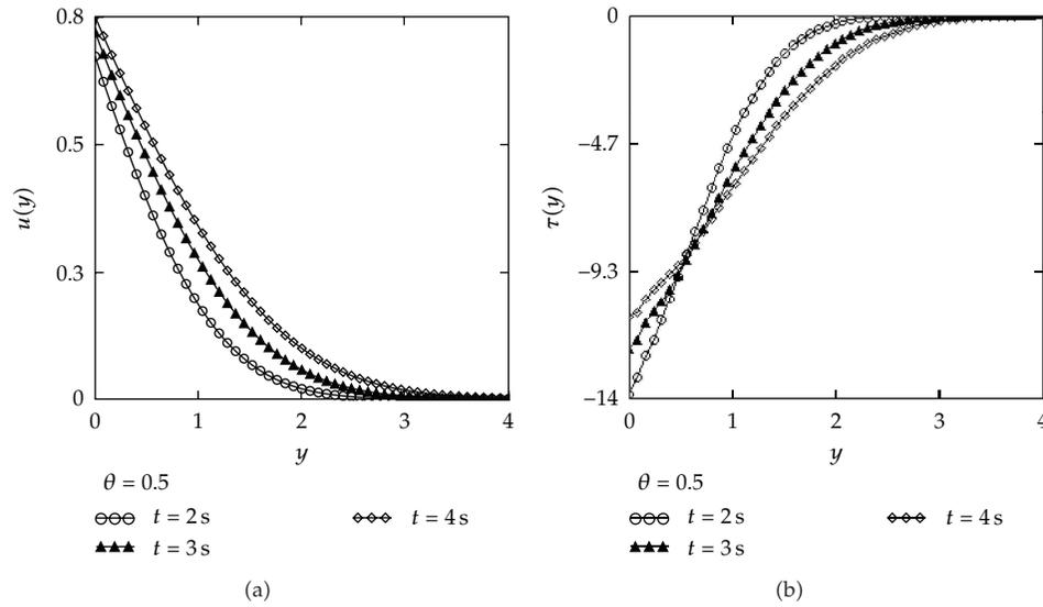
**Figure 1:** Profiles of the velocity field  $u(y, t)$  and the shear stress  $\tau(y, t)$  for fractional Maxwell fluid given by (4.7) and (4.15), for  $U = 1$ ,  $y = 1$ ,  $\nu = 0.379$ ,  $\mu = 33$ ,  $\lambda = 1.5$ ,  $\alpha = 0.2$ ,  $\theta = 0.5$ , and different values of  $t$ .
