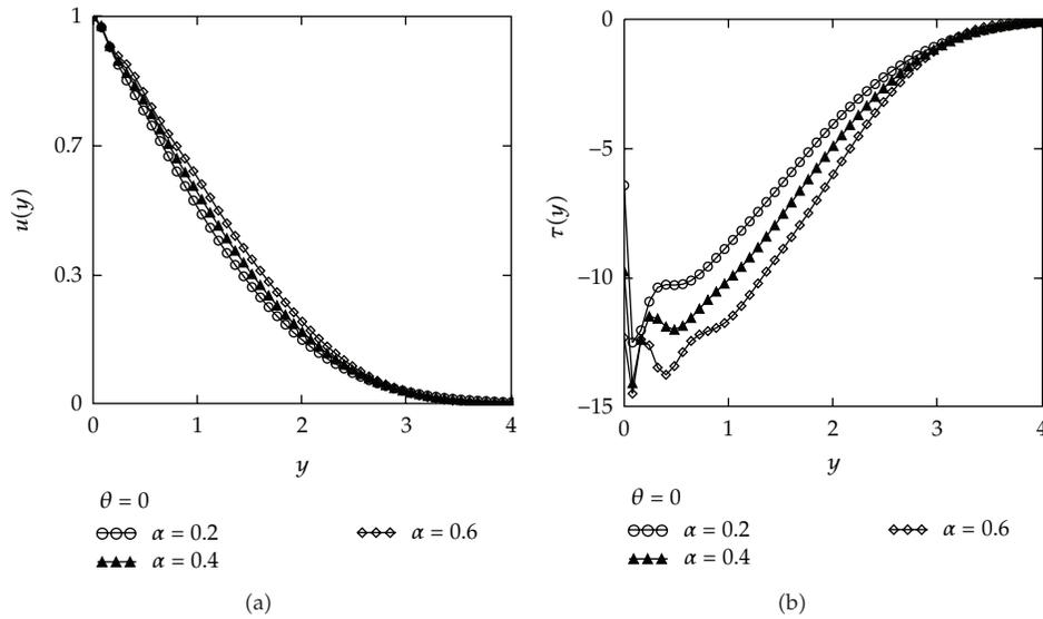
**Figure 8:** Profiles of the velocity field  $u(y,t)$  and the shear stress  $\tau(y,t)$  for fractional Maxwell fluid given by (5.3) and (5.4), for  $U = 1, y = 1, \nu = 0.379, \mu = 33, \lambda = 1.5, \theta = 0.0, t = 5$  s, and different values of  $\alpha$ .
