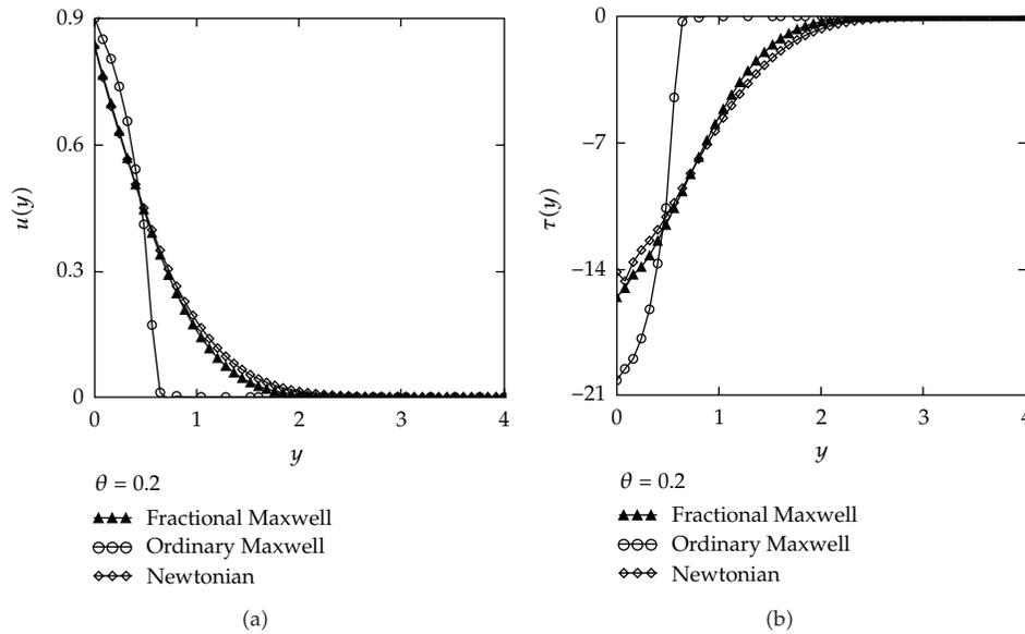
**Figure 13:** Profiles of the velocity field  $u(y,t)$  and the shear stress  $\tau(y,t)$  for fractional Maxwell, ordinary Maxwell and Newtonian fluids, for  $U = 1$ ,  $y = 1$ ,  $\nu = 0.379$ ,  $\mu = 33$ ,  $\lambda = 1.5$ ,  $\alpha = 0.2$ ,  $t = 2$  s, and  $\theta = 0.2$ .
