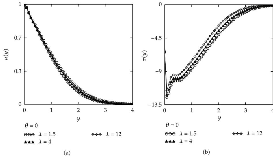
**Figure 6:** Profiles of the velocity field  $u(y,t)$  and the shear stress  $\tau(y,t)$  for fractional Maxwell fluid given by (5.3) and (5.4), for  $U = 1, y = 1, \nu = 0.379, \mu = 33, \alpha = 0.2, \theta = 0.0, t = 5$  s, and different values of  $\lambda$ .
