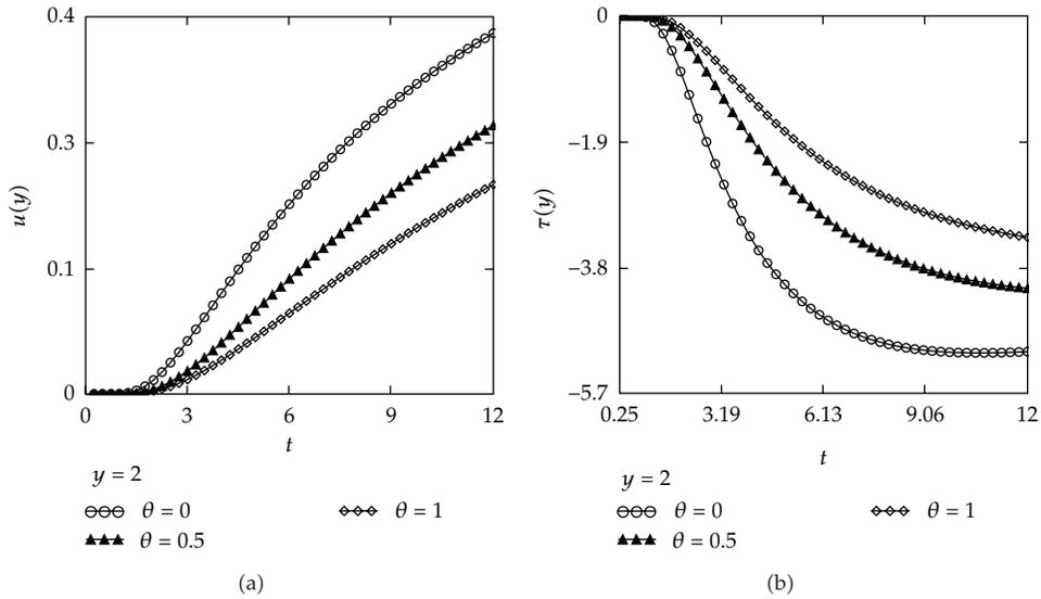
**Figure 4:** Profiles of the velocity field  $u(y,t)$  and the shear stress  $\tau(y,t)$  for fractional Maxwell fluid given by (4.7) and (4.15), for  $U = 1$ ,  $y = 2$ ,  $\nu = 0.379$ ,  $\mu = 33$ ,  $\lambda = 1.5$ ,  $\alpha = 0.2$ , and different values of  $\theta$ .
