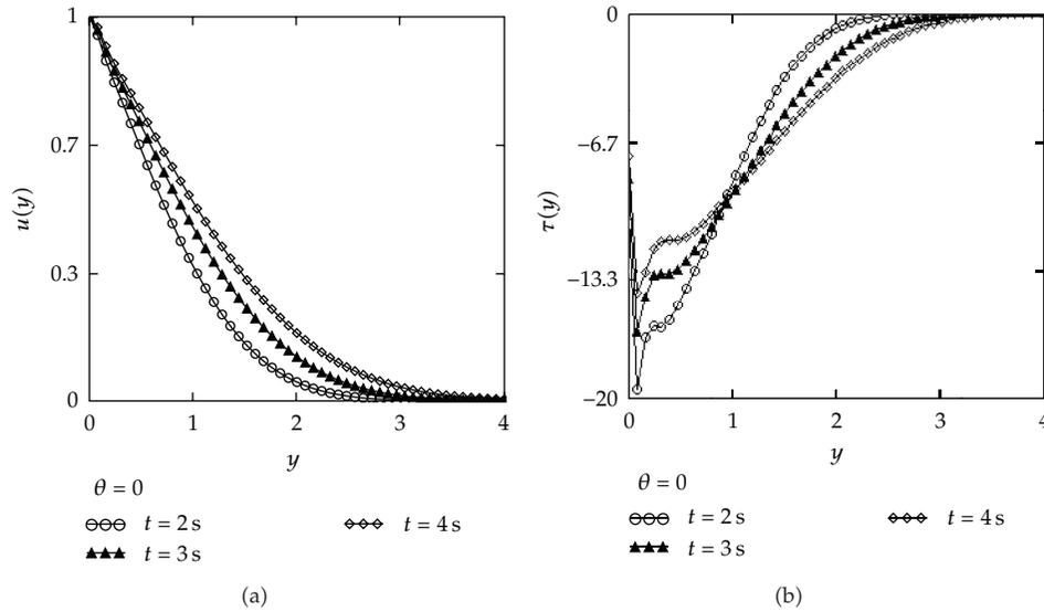
**Figure 2:** Profiles of the velocity field  $u(y,t)$  and the shear stress  $\tau(y,t)$  for fractional Maxwell fluid given by (5.3) and (5.4), for  $U = 1, y = 1, \nu = 0.379, \mu = 33, \lambda = 1.5, \alpha = 0.2, \theta = 0.0$ , and different values of  $t$ .
