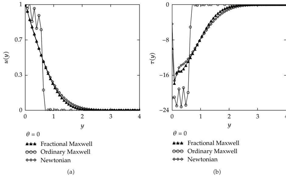
**Figure 12:** Profiles of the velocity field  $u(y,t)$  and the shear stress  $\tau(y,t)$  for fractional Maxwell, ordinary Maxwell and Newtonian fluids, for  $U = 1$ ,  $y = 1$ ,  $\nu = 0.379$ ,  $\mu = 33$ ,  $\lambda = 1.5$ ,  $\alpha = 0.2$ ,  $t = 2$  s, and  $\theta = 0.0$ .
