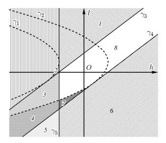
**Figure 3.** The bifurcation diagram in the Lagrange's problem on the pseudosphere. The domain of prohibited motion is shaded by the vertical lines while the domains of possible motion are denoted by the numbers
