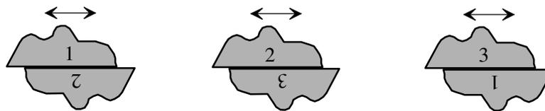
Figure 1.4. Grinding flat mirrors.
