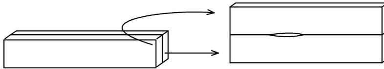
Figure 1.3. Carpenter's method for checking straightness.
