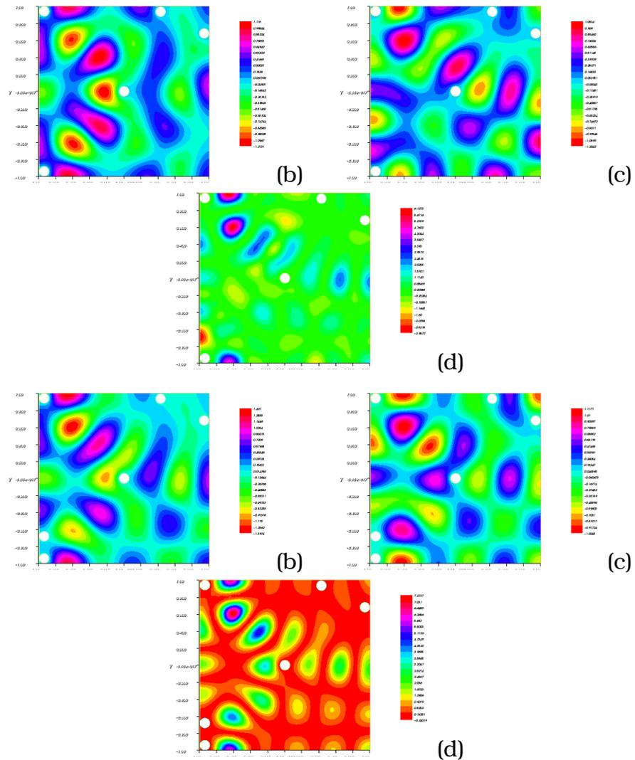
FIGURE 20. FIRST STEP: b)DIRECT STATE, c)ADJOINT STATE d)TOPOLOGICAL DERIVATIVE. First step: b)Direct State, c)Adjoint state d)Topological derivative
