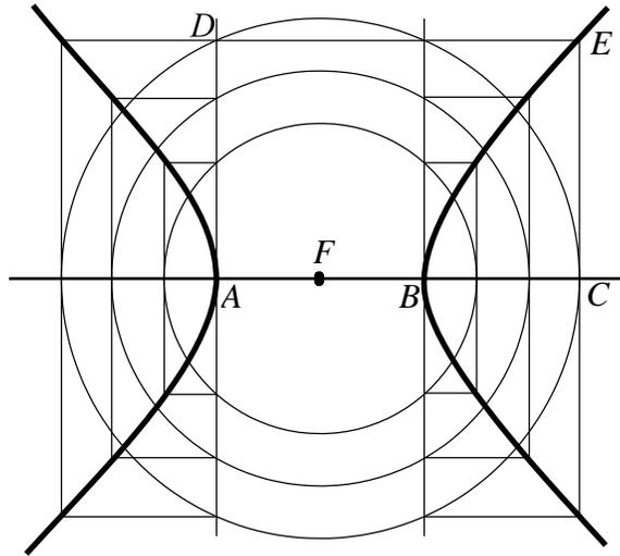
Figure 19.8 Construction of hyperbola
