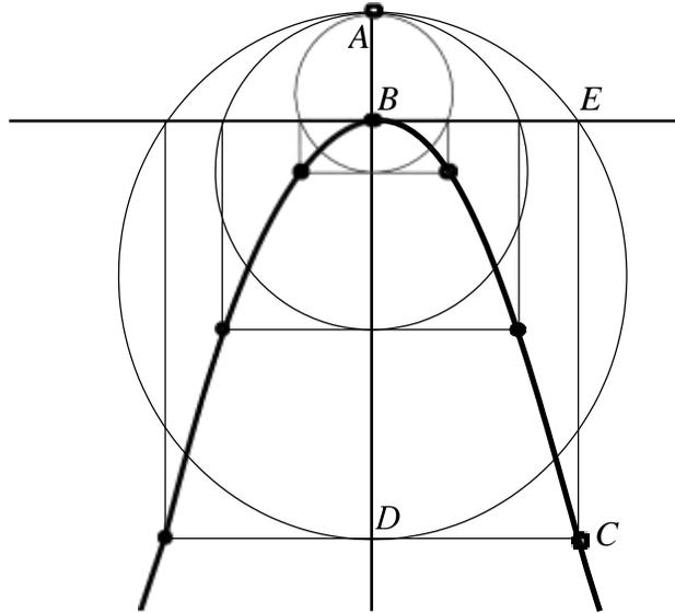
Figure 19.6 Construction of parabola
