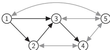
Fig. 12.2. A graph that can be decomposed only after removing the sink node 5.
