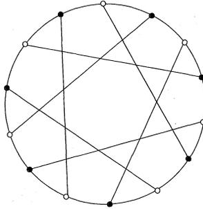
This graph (which has 14 vertices and 21 edges) is the incidence graph of the projective plane over the field  $F_2$  of two elements, namely the Fano plane  $P^2F_2$ .
