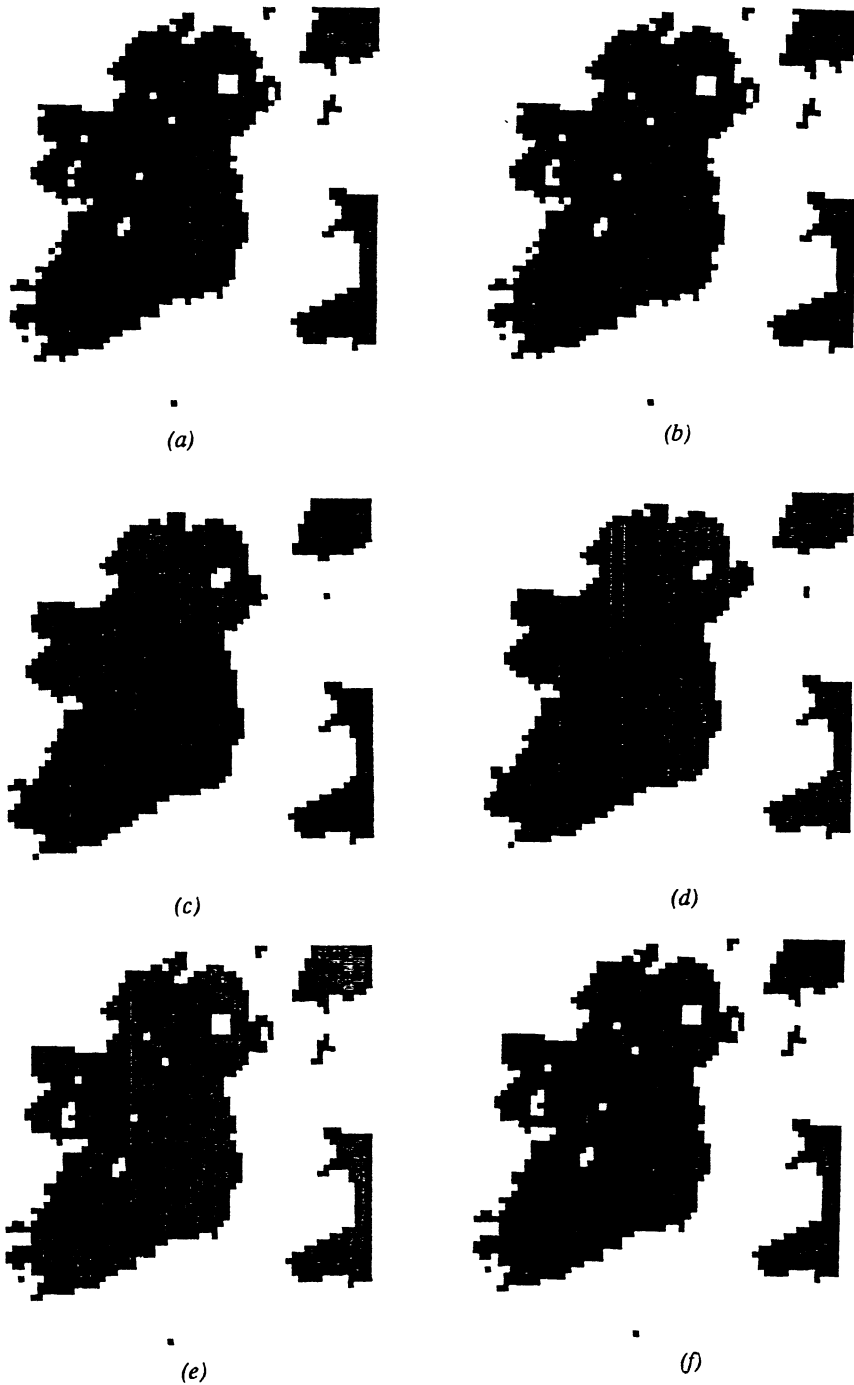
Figure 5. Restorations at 64 \times 64 pixels. Left column MAP, right column MMP. Rows are 8 neighbours, \beta = 0.7 , 8 neighbours, \beta = 2.0 , 4 neighbours, \beta = 1.4 , and 4 neighbours, \beta = 4.0 .
