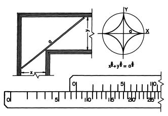
The rule is set for x = 8. From it we read that if y = 10 then a = 25.3; anything shorter than this will pass around the corner. If the girder is 20 feet long and x = 8feet then the second corridor must be about 6.1 feet wide in order that the girder can make the turn.
