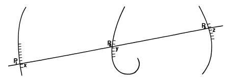
We lay a straight line across the figure, cutting the scales at the points  $P_1, P_2, P_3$ , with scale readings x, y, z. The coordinates of the points, namely,  $(X_1, Y_1)$ ,  $(X_2, Y_2)$ ,  $(X_3, Y_3)$  respectively, are given by Equations (4).
