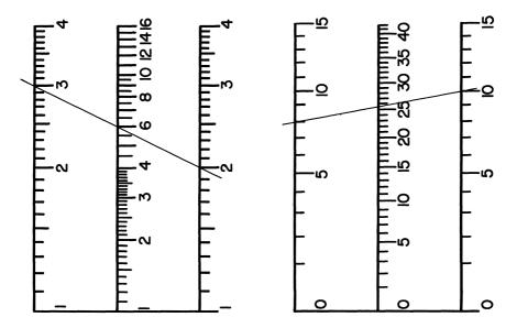
A chart for multiplication which does not employ logarithmic scales can be devised. The equation
