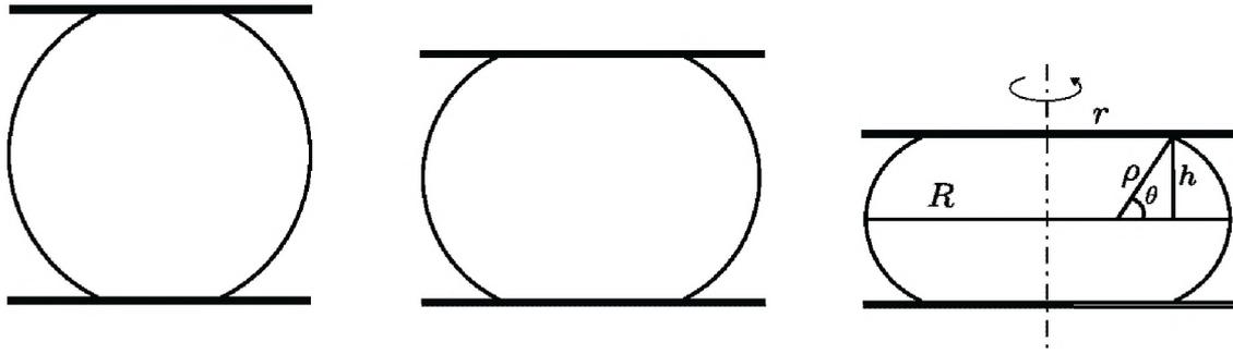
Figure 1: Geometry of Cole's experiment. The shown profiles are obtained using the linear approximations  $R(m) = 1.64a - 0.68ma$ ,  $\rho(m) = 1.12ma$  and different values of the deformational parameter  $m \in (0, 1]$ .
