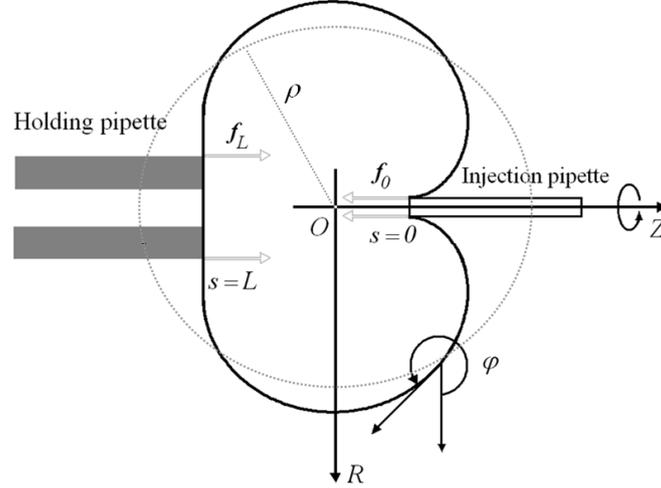
**Figure 1.** Sketch of an initially spherical cell membrane of radius  $\rho$  deformed axisymmetrically by two micro-pipettes in the process of a micro-injection. Here,  $Z$ -axis is the symmetry axis of the cell,  $\varphi$  is the slope angle of the profile curve, which is assumed to lie in the  $ROZ$ -plane while  $f_0$  and  $f_L$  are the magnitudes of the forces (per unit contour length) exerted by the micro-pipettes at the contours  $s = 0$  and  $s = L$ .
