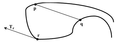
Figure 2.13. Mean Value Theorem for Plane Curves.
