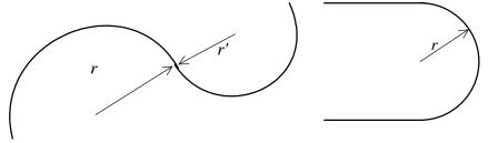
Figure 2.6. Curvature need not vary continuously.
