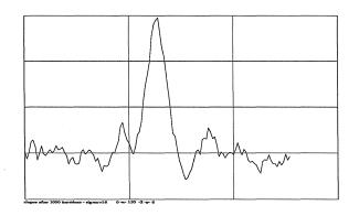
Figure 3: Reconstructed  $1^{st}$  Derivative - 1000 iterations After 1000 iterations, the smoothness in the reconstructed function is reflected by the present estimate of slopes. The slope of the original step edge clearly dominates.
