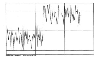
Figure 1: Step edge corrupted with guassian noise  $\sigma = 16$ Original data of 128 samples. The step edge has been corrupted by additive gaussian noise of standard deviation sigma = 16.
