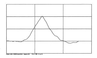
Figure 6: Reconstructed  $1^{st}$  Derivative - 10000 iterations After 10000 iterations, the step edge is clearly visible in the dominant peak of the first derivative. Smoothing has considerably broadened this peak, however.
