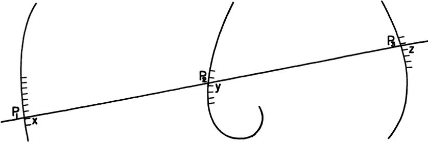
We lay a straight line across the figure, cutting the scales at the points  $P_1, P_2, P_3$ , with scale readings  $x, y, z$ . The coordinates of the points, namely,  $(X_1, Y_1)$ ,  $(X_2, Y_2)$ ,  $(X_3, Y_3)$  respectively, are given by Equations (4).
