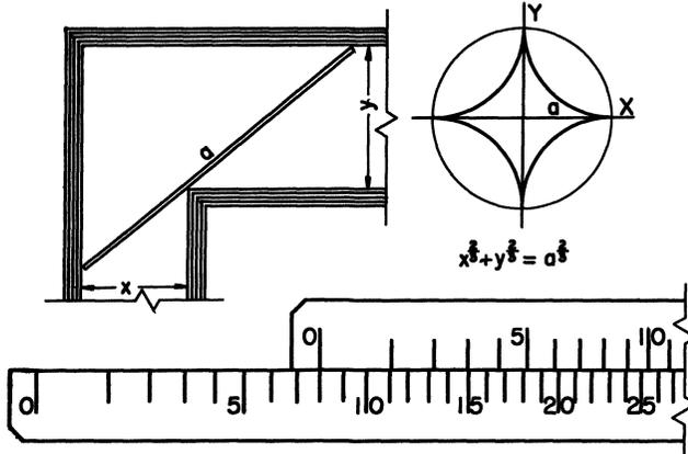
The rule is set for  $x = 8$ . From it we read that if  $y = 10$  then  $a = 25.3$ , anything shorter than this will pass around the corner. If the girder is 20 feet long and  $x = 8$  feet then the second corridor must be about 6.1 feet wide in order that the girder can make the turn.
