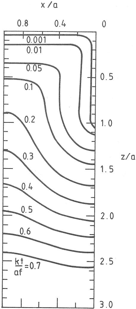
Figure 3. Development of the wetting front with dimensionless time  $Kt/af$  when  $\psi_c/a = -1.0$  and  $b/a = 1.0$ .
