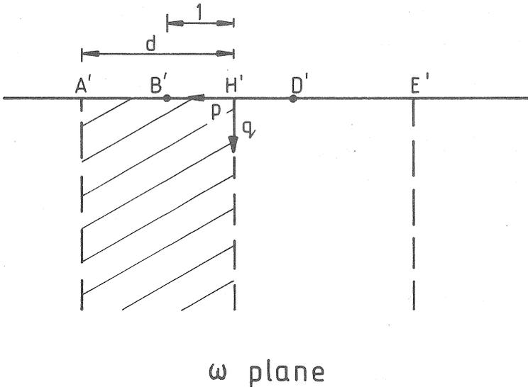
Figure 2. Representation in the transformed ( $\omega$ ) plane of a soil which contains regularly spaced vertical cracks in the physical plane. The broken lines are line of symmetry and the width of the shaded region is half a period.
