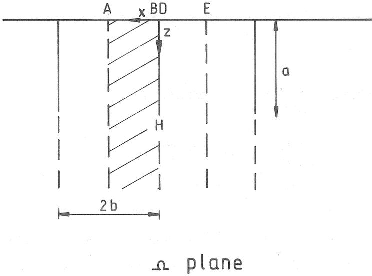
Figure 1. Representation in the physical ( $\Omega$ ) plane of a soil containing regularly spaced vertical cracks of depth  $a$  and spacing  $2b$ . The broken lines are lines of symmetry and the width of the shaded region is half a period.
