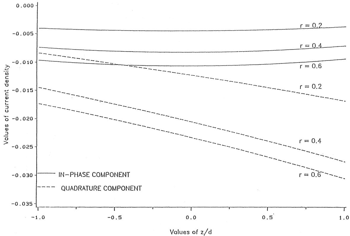
Figure 2. Current density variation across the thickness of the sheet at three different values of  $r$ .  $\alpha = 1$ ,  $\lambda = 1$  and  $\delta = 0.1$ .
