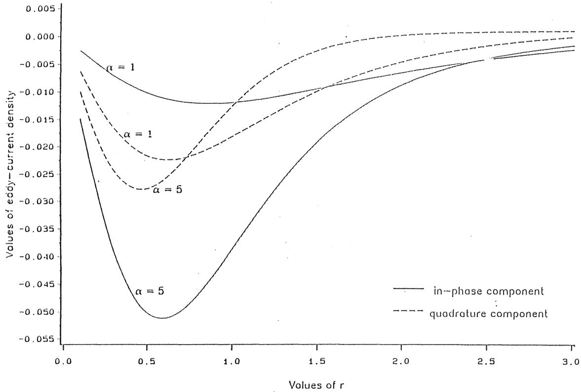
Figure 1. Zeroth order current density,  $j_0^{(0)}$ , as a function of  $r$  for  $\alpha = 1$  and  $5$ .
