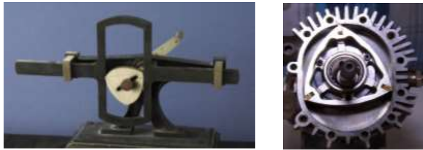
Figure 21.8 Mechanisms utilizing a Reuleaux triangle: Reuleaux model and rotary (Wankel) engine
