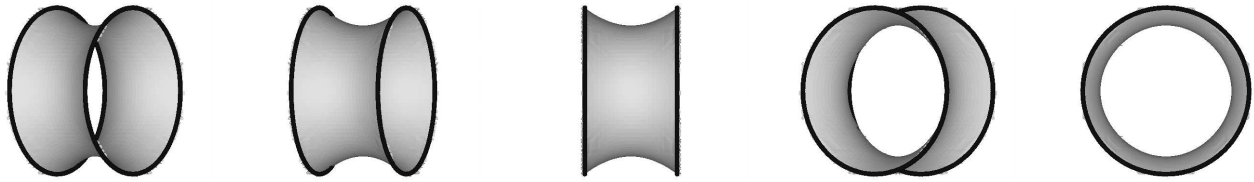
FIGURE 13. Catenoid spanning rings of radius .5 and separated by the distance 2 \times .277259 . The initial approximation was a cylinder. The mesh used had step 0.025 along each coordinate, and its size was 27 \times 47 \times 47 .
