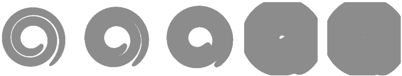
FIGURE 3. Spiral “flame” spreading under F(\kappa) = 1 - .1\kappa . The initial curve (not shown) and the grid are the same as in Figure 2. As the spiral expands, it separates into two flames (boundary components), one propagating outwards and one inwards. The inner front collapses and disappears, and all that remains is the outer front, which asymptotically approaches a circle.
