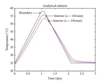
FIGURE 5: The interior temperatures calculated by the analytical solution (at x = 150 mm and x = 250 mm).
