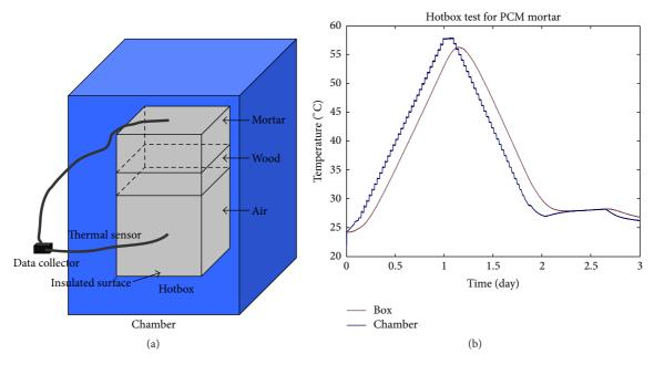
FIGURE 4: A heat conduction test: (a) experimental setup; (b) test results [8].
