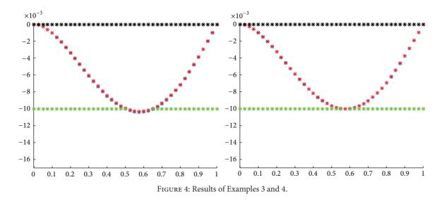
Gao beam: maximal deflection -0.0094 m, contact zone:  $\emptyset$ .
