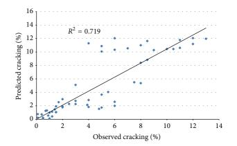
FIGURE 2: Comparison between predicted and observed cracking values based on the out of sample data.
