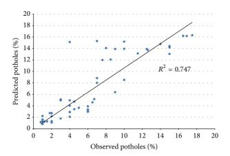
FIGURE 3: Comparison between predicted and observed pothole values based on the out of sample data.
