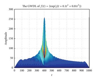
FIGURE 2: *t*-amplitude distribution of QFM signal in GWDL domain.
