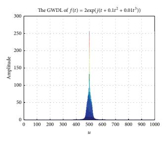
FIGURE 3: *u*-amplitude distribution of QFM signal in GWDL domain.
