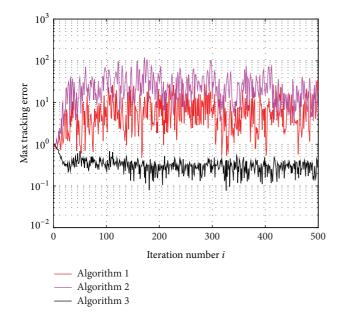
FIGURE 2: The max tracking error versus iteration with 5% packet dropout.
