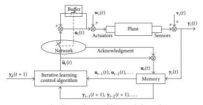
FIGURE 1: The schematic diagram of the networked control system.
