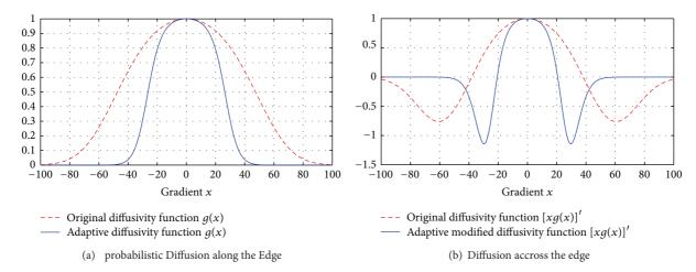
FIGURE 1: The Adaptive probabilistic diffusivity function  $g_{apr}()$  versus the original probabilistic diffusivity function  $g_{pr}()$ . (a) Diffusivity functions along the edge (g(x)). (b) Diffusivity functions across the edge ([xg(x)]').
