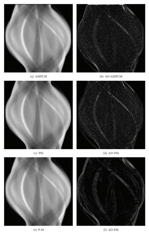
Figure 5: Mean of the filtered sinograms (left column). Absolute difference between the mean of the filtered sinograms and the noise-free image (right column).
