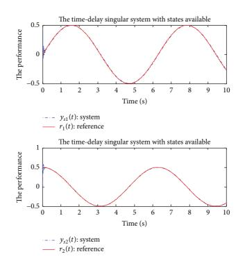
FIGURE 3: Output responses of time-delay singular system with states available by the new digital redesign approach.
