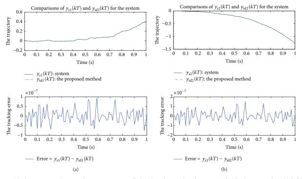
FIGURE 7: (a) The comparison between the system output  $y_{s1}(kT)$  and its observer-based output  $y_{id1}(kT)$  by the proposed method. (b) The comparison between the system output  $y_{s2}(kT)$  and its observer-based output  $y_{id2}(kT)$  by the proposed method.
