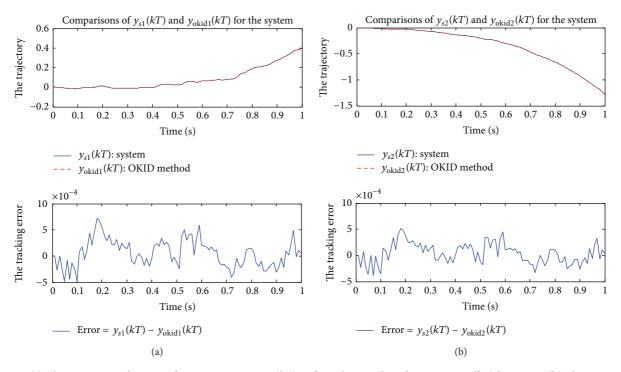
FIGURE 6: (a) The comparison between the system output  $y_{s1}(kT)$  and its observer-based output  $y_{okid1}(kT)$  by OKID. (b) The comparison between the system output  $y_{s2}(kT)$  and its observer-based output  $y_{okid2}(kT)$  by OKID.
