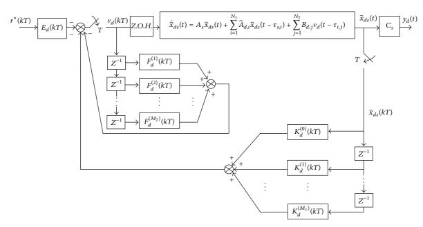
FIGURE 1: Digital redesign for time-delay singular system.
