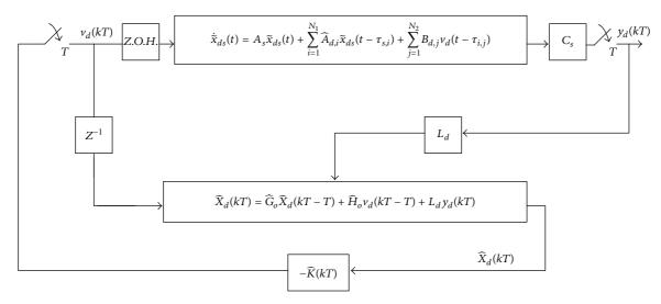
FIGURE 2: Observer-based suboptimal tracker for the digitally redesigned time-delay singular system.
