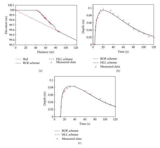
**Figure 3:** Comparisons with WES experiment: (a) water surface profile along the channel at  $t = 10 \,\text{sec}$ ; (b) time evolution of water depth at  $x = 70.1 \,\text{m}$ ; (c) time evolution of water depth at  $x = 85.4 \,\text{m}$ .
