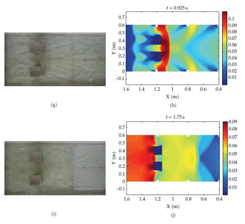
**Figure 5:** Comparisons of experiments and numerical simulations—(a) and (b) when t = 0.56 sec, dambreak flow arrives to the columns; (c) and (d) when t = 0.625 sec, dam-break flow moves to the middle of the columns; (e) and (f) when t = 0.725 sec, dam-break flow surrounds the columns and forms vortexes; (g) and (h) when t = 0.925 sec, dam-break flow touches the boundary of tank; (i) and (j) when t = 1.75 sec, the flow returns to the location of gate.
