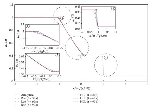
**Figure 2:** Increasing accuracy by decreasing the grid size to  $\Delta x = 2$  m.
