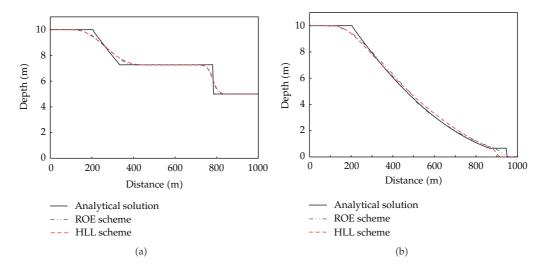
**Figure 1:** Idealized dam-break problem: (a) initial depth ratio  $H_r/H_t = 2$ ; (b) initial depth ratio  $H_r/H_t = 1000$
